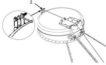
Guide the Cord over the bin roof (as pictured above) and use the Self- Drilling Screws to attach the Cord Retainer to the edge of the bin roof (as pictured below). 2 large holes on the Cord Retainer are provided to allow the bin bolts to pass through. (as pictured below)
