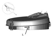
Wrap end of the Cord around the bolt and tie securely. KNOT MUST BE TIGHT TO SECURE CORD. (as pictured below)
